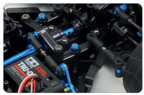
The kit comes with a hi-torque servo saver as standard, to help protect the servo and steering linkage from damage.
