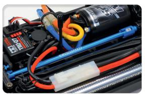
An aluminum propeller shaft is joined by propeller joints designed specially for use with the included plastic anti-wear caps.
