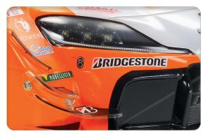
The head light case is painted black. The lower 2 sheets are fixed to the body with screws as one part.
