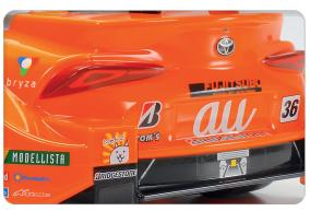
The flat upper part of the trunk, the box shape of the rear part of the fender, the diffuser, etc.
